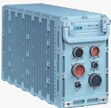
The removable front panel and top and bottom covers simplify maintenance of circuit cards, power supply and backplane I/O wiring.
