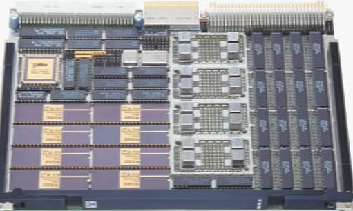
This universal serial module supports standard communication protocols up to 5 Mbs. BIT capabilities even allow testing on-board transceivers.
