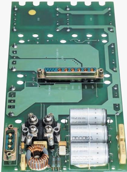
All power supplies are full military class and incorporate new generation DC/DC converters with up to 90% efficiency. Nominal input voltages are 115 VAC and 28 VDC according to MIL-STD-704.
