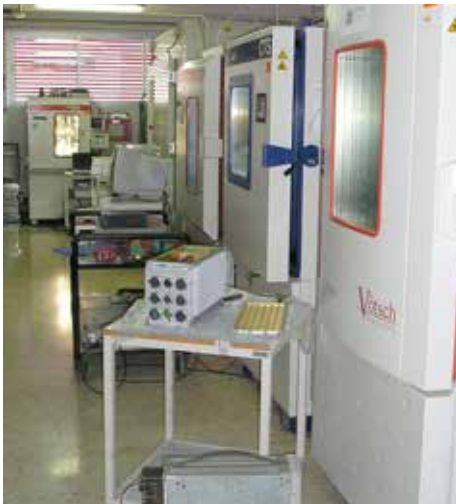
THE CM-ATR HAS PASSED HIGH TEMPERATURE OPERATION TEST. CONSTANT TEMPERATURE EXPOSURE WAS 80 °C (MAX. REACHED WAS 93.8 °C).
