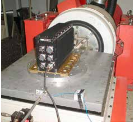
THE CM-ATR PASSES VIBRATION TEST (AXIS X CONFIGURATION), 12 grms @15 to 2000 Hz, NO SHOCK ABSORBERS, 1 HOUR PER AXIS.
