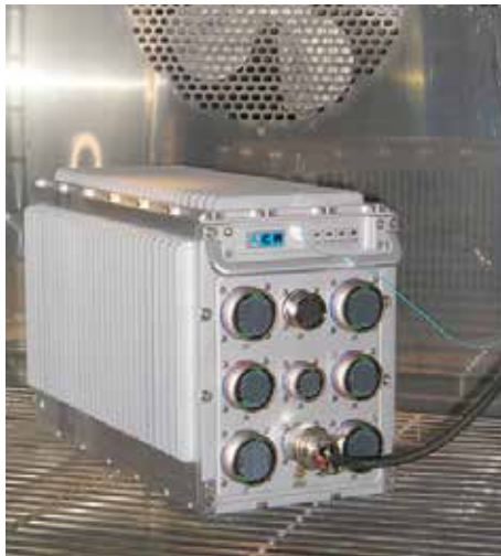
THE CM-ATR PASSES HIGH TEMPERATURE STORAGE TEST. CONSTANT TEMPERATURE EXPOSURE WAS 100 °C.
