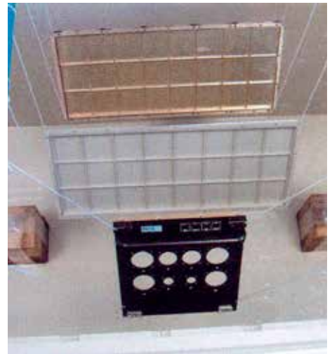
THE CM-ATR PASSES SALT FOG TEST (PHOTO 1), TEST OF 96 HOURS. SALT SOLUTION OF 5% NaCl pH 6.30.
