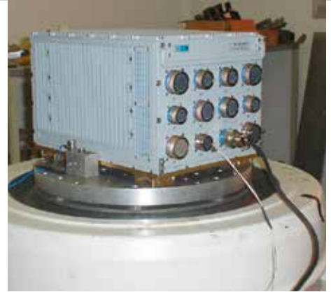
THE CM-ATR PASSES SHOCK TEST (AXIS Z CONFIGURATION), SAWTOOTH PULSE 20 grms @11 ms, 18 SHOCK PER AXIS, NO SHOCK ABSORBERS.
