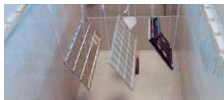
THE CM-ATR PASSES HIGH TEMPERATURE STORAGE TEST. CONSTANT TEMPERATURE EXPOSURE WAS 100 °C.
