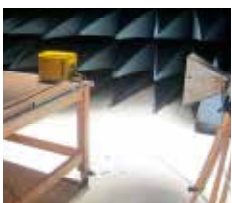
THE CM-ATR-3U PASSES ELECTROMAGNETIC RADIATED SUSCEPTIBILITY, MAGNETIC FIELD, 30HZ. MIL-STD-461F CERTIFICATE AVAILABLE.
