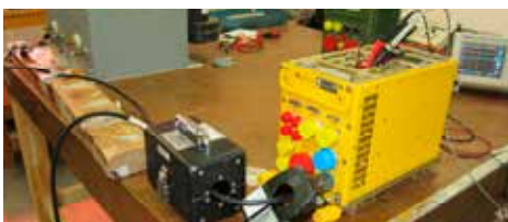
THE CM-ATR-3U PASSES ELECTROMAGNETIC RADIATED SUSCEPTIBILITY, MAGNETIC FIELD, 30HZ. MIL-STD-461F CERTIFICATE AVAILABLE.
