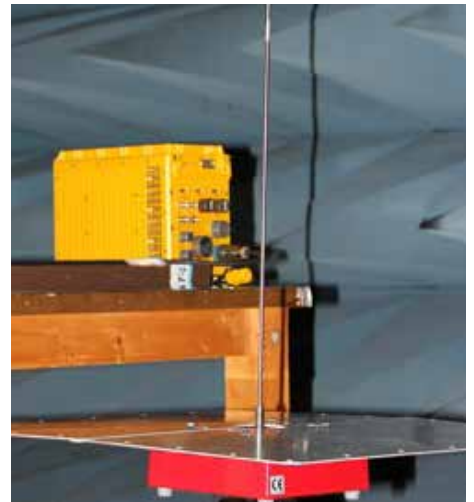
THE CM-ATR-3U PASSES ELECTROMAGNETIC EMISSION & RADIATION TEST. RADIATED E FIELD 2 MHz to 30 MHz. MIL-STD-461F CERTIFICATE AVAILABLE.
