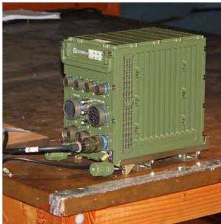
THE CM-ATR-3U PASSES ELECTROMAGNETIC IMMUNITY TEST. CONDUCTED SUSCEPTIBILITY DAMPED SINUSOIDAL TRANSIENTS, CABLES AND POWER LEADS 10 KHz to 100 MHz. MIL-STD-461F CERTIFICATE AVAILABLE.
