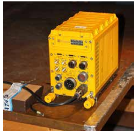
THE CM-ATR-3U PASSES ELECTROMAGNETIC IMMUNITY TEST. CONDUCTED SUSCEPTIBILITY DAMPED SINUSOIDAL TRANSIENTS, CABLES AND POWER LEADS 10 KHz to 100 MHz. MIL-STD-461F CERTIFICATE AVAILABLE.
